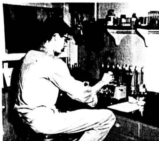
DAVID DAVIS, sophomore chemical technology student, runs a sedimentation test to determine quality of protein in wheat.
